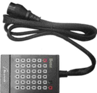
Figure 1.35 Mercedes Benz pin board (38P)
