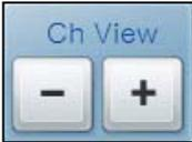
: 5 current data are displayed on the screen at once by default. The number of data displayed on the screen can be set from 1 to 8.
