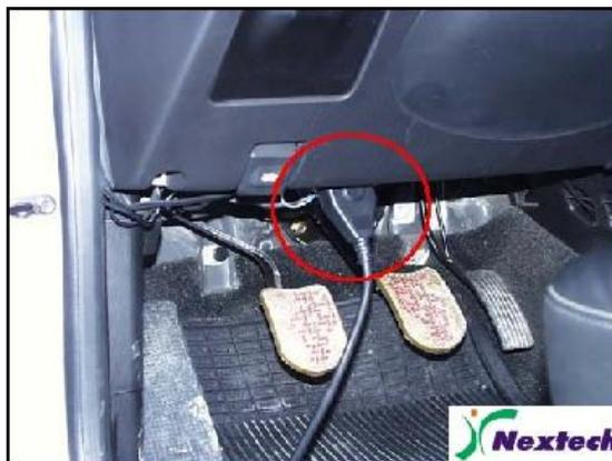
**Figure 8.1 OBD-II Diagnostic connector location**
