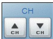
: In the graph screen, up to 8 current data are displayed at once. If more than 8 current data are saved, click the channel ▲ and ▼ keys to scroll the current data.
