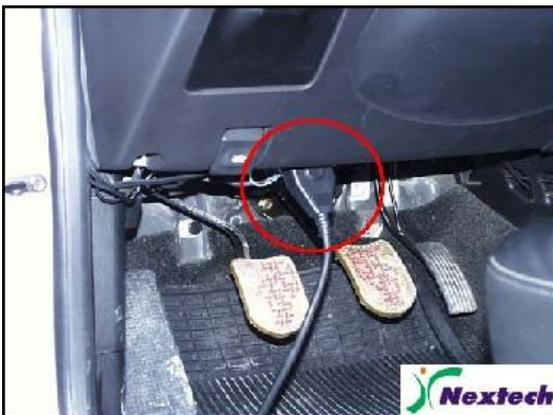
**Figure 6.1** Location of OBD-II diagnostic connector
