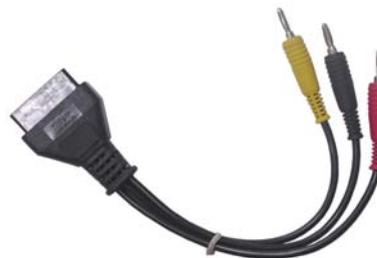
Figure 1.38 Mercedes Benz Cable (3 liners)
