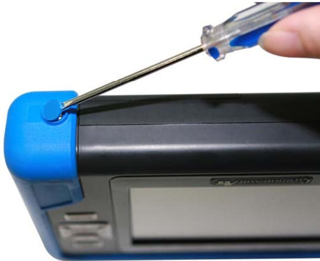
3. Remove the screw using the driver.
