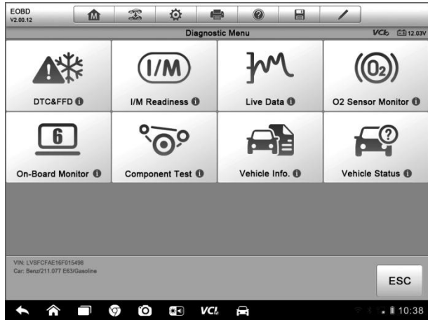
Figure 4-18 Sample OBD II Diagnostic Menu
