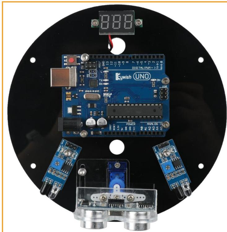
Figure 3.1.8.2 Effect diagram of voltage display module installation
