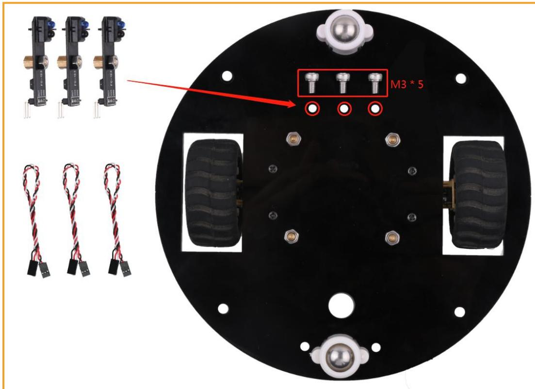
Figure 3.1.4.2 Schematic diagram of the tracing module installation
