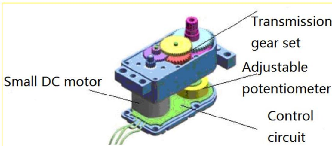
Figure . 3. 2. 4. 1 Diagram of Steering Gear
