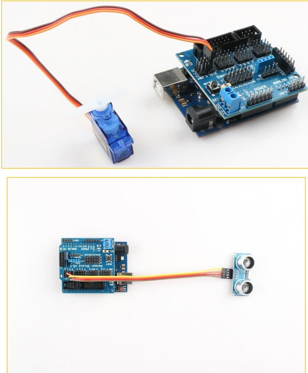
Figure .3.2.4.8 Wiring of the Steering Gear and Ultrasonic Module
