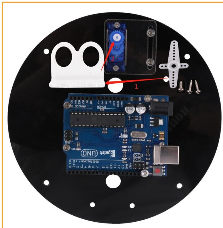
**Note: Firstly, use the rudder paddle to fix the ultrasonic bracket**
