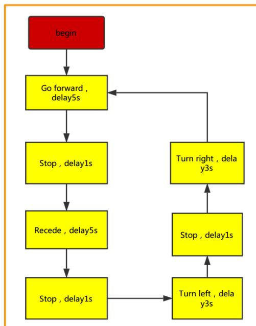
Figure 3.1.2.9 Motor Test Flow Chart
