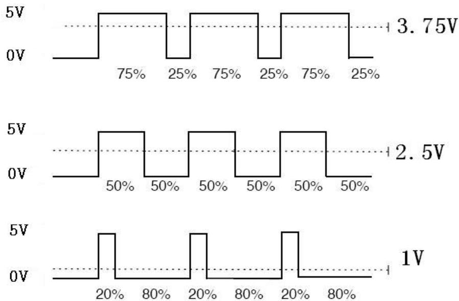
Figure 3.2.1.6Relation between Pulse and Voltage
