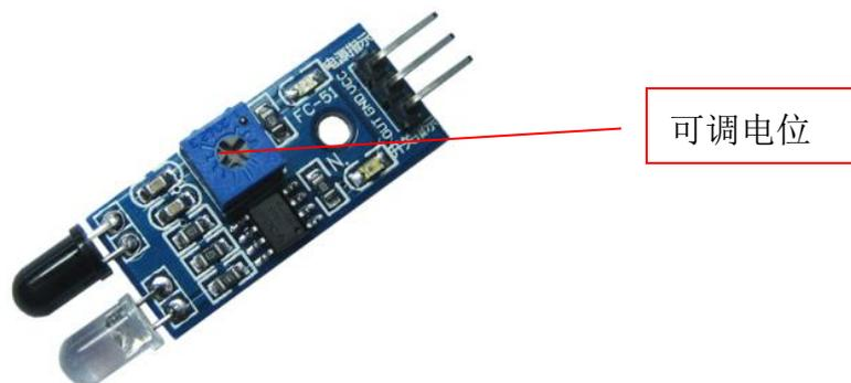
Figure .3.2.2.4 Diagram of Distance Detection Adjustment
