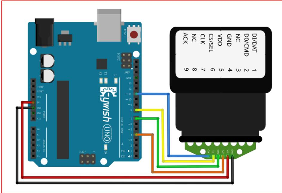
Figure 3.2.7.5 Connection of Arduino and Receiving Head Wires
