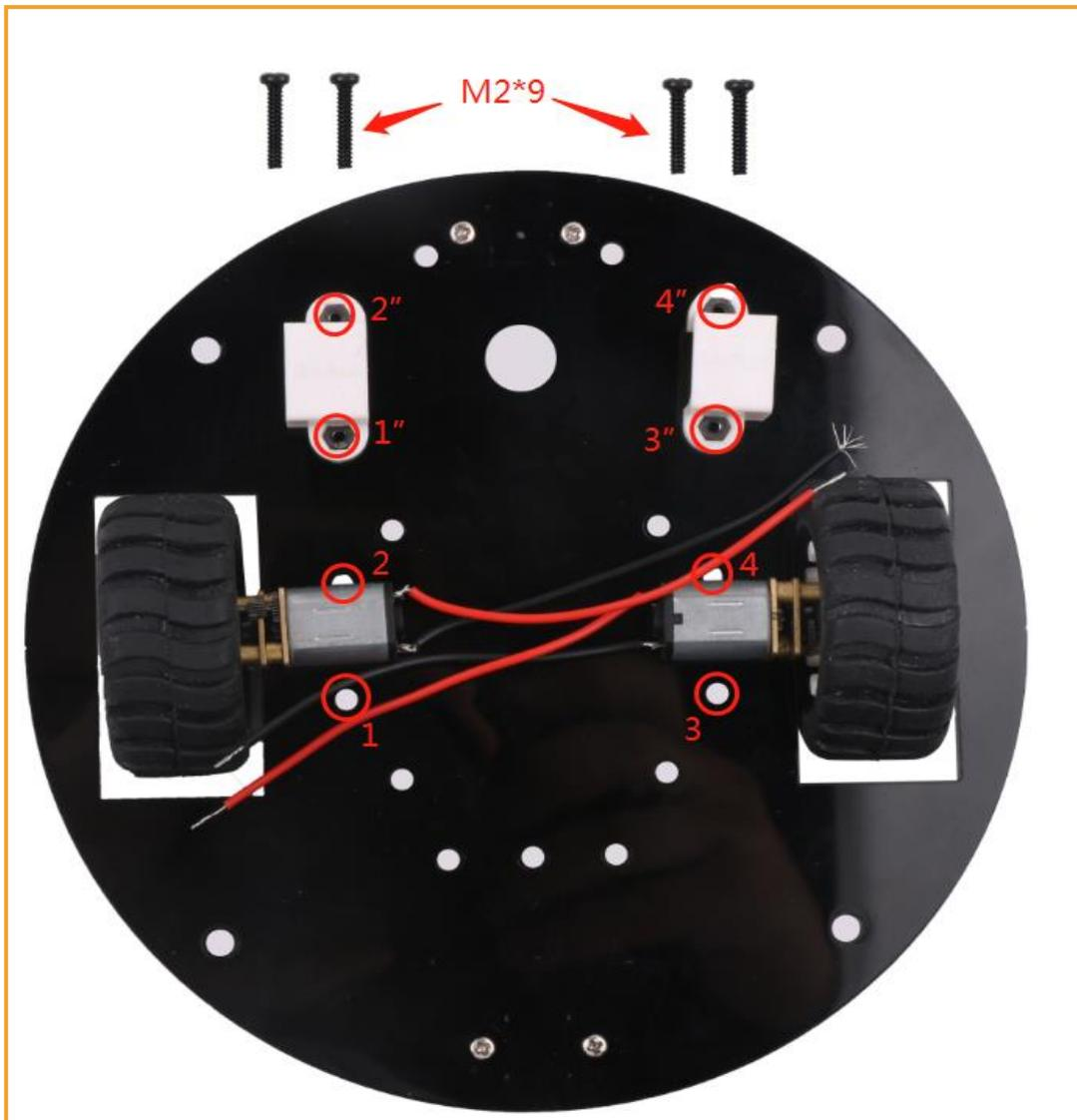
**Note: Hole 1 corresponds to the nut 1", tightened from the bottom with an M2\*9 Phillips screw, and so on.**
