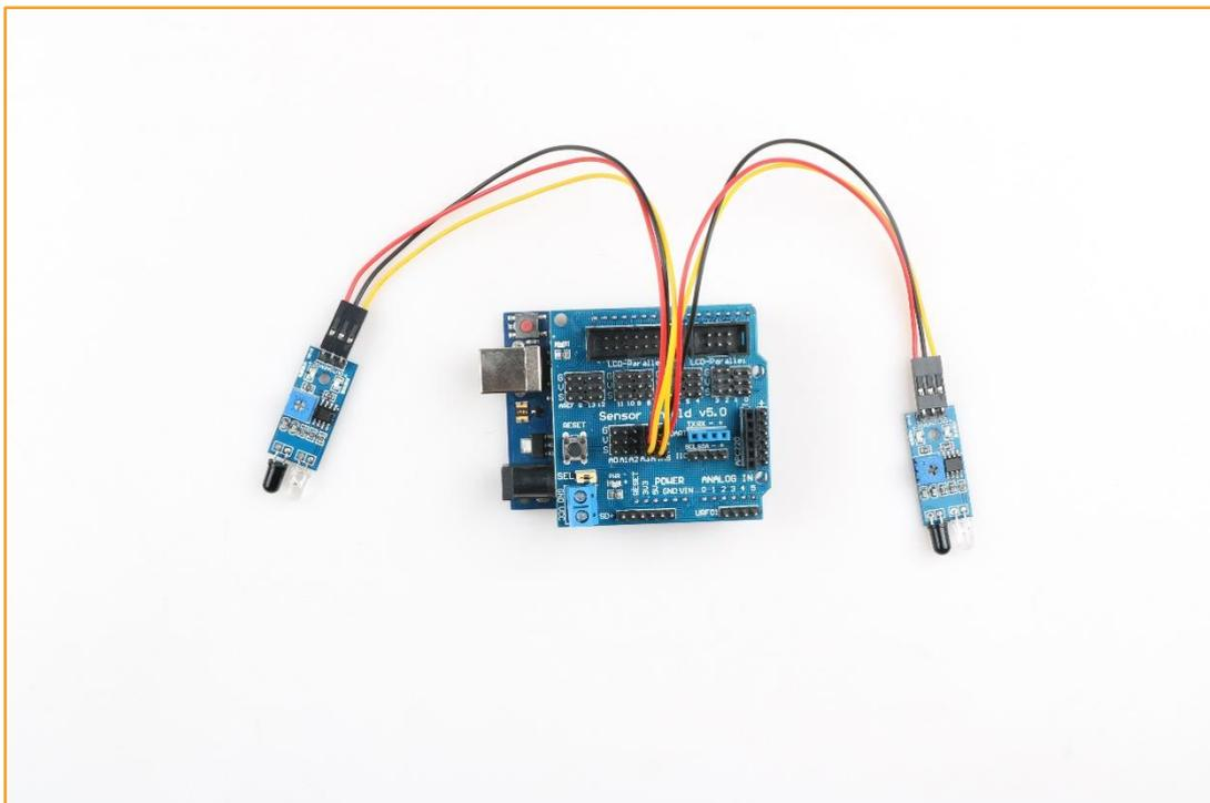
Figure 3.1.7.3 Wiring diagram of infrared obstacle avoidance module
