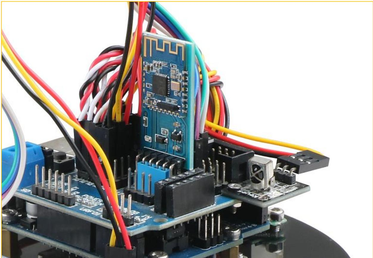
Figure .3.2.6.4 Installation of Bluetooth Module
