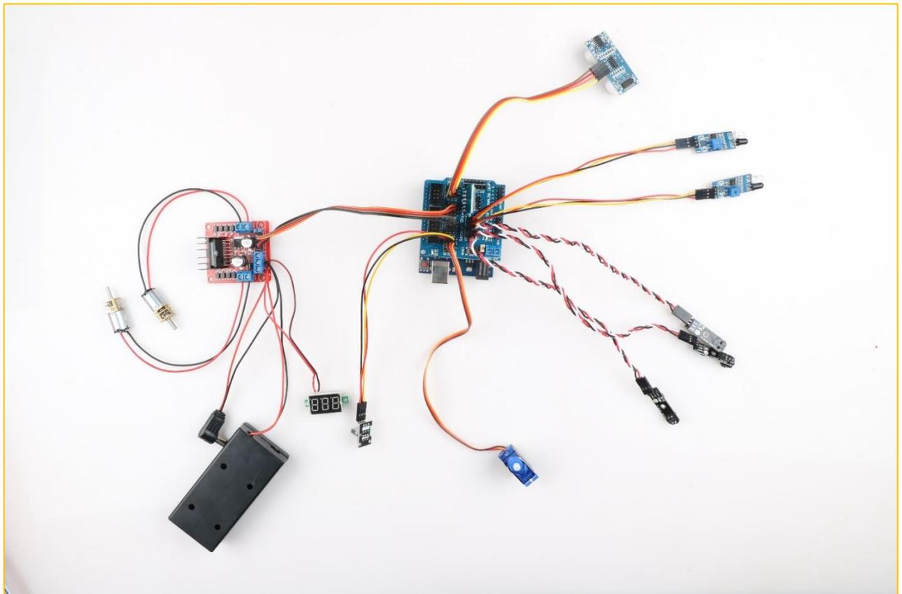
Figure 3.1.2.7 Arduino and L298N driver board connection diagram and connection table
