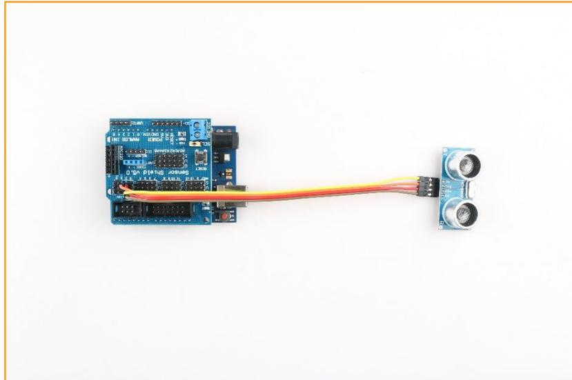
Figure 3.1.6.10 Diagram of ultrasonic connection
