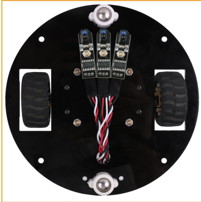
Figure 3.1.4.3 Effect diagram of the tracing module installation
