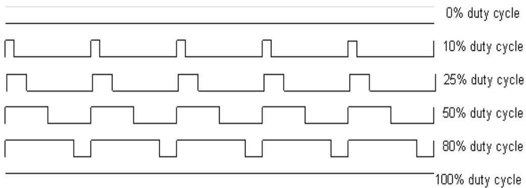
Figure .3.2.1.5 Sequence Diagram of PWM Duty Cycles
