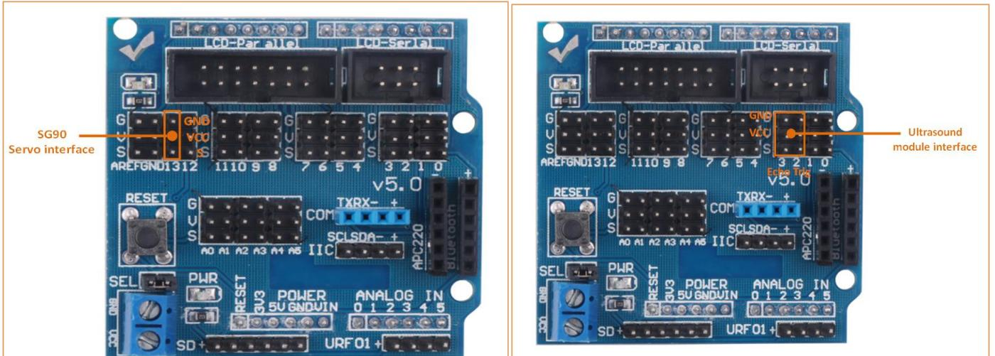
Figure 3.2.4.9 Wiring diagram of steering gear, ultrasonic wave and expansion board
