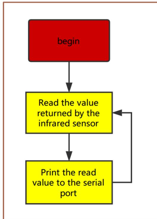
Note: Here we connect the signal output port of infrared obstacle avoidance to the analog port on Arduino (A0-A5), so the serial port monitor prints analog values, you can connect it to the digital port (2-13), then the serial port monitor will print out only "0" and "1".
