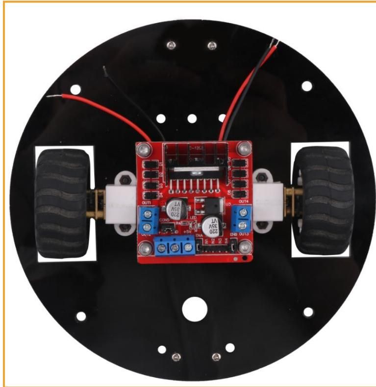
Figure 3.1.3.4 Effect diagram of Motor Driver Board Installation
