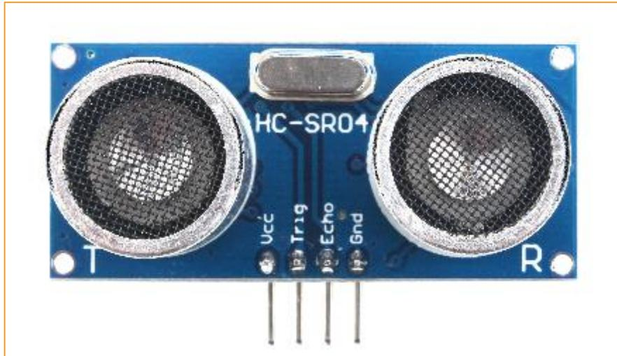
Figure 3.2.4.3 Physical Map of Ultrasonic Module
