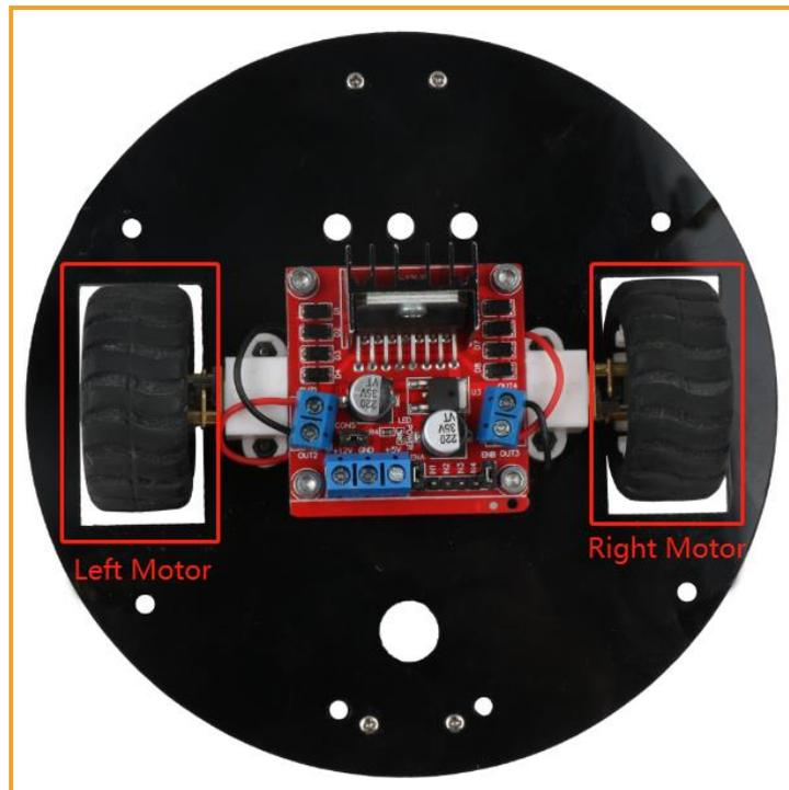
Note: The left motor positive pole is connected to OUT1, the negative pole is connected to OUT2; the right motor positive pole is connected to OUT3, and the negative pole is connected to OUT4.
