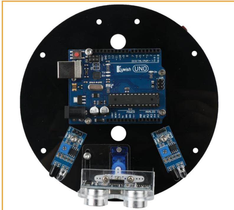
Figure 3.1.7.2 Effect diagram of infrared obstacle avoidance module installation
