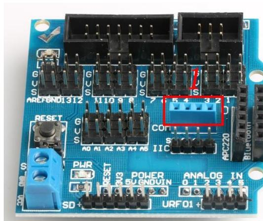
Figure .3.2.6.3 Wiring Positions of Bluetooth
