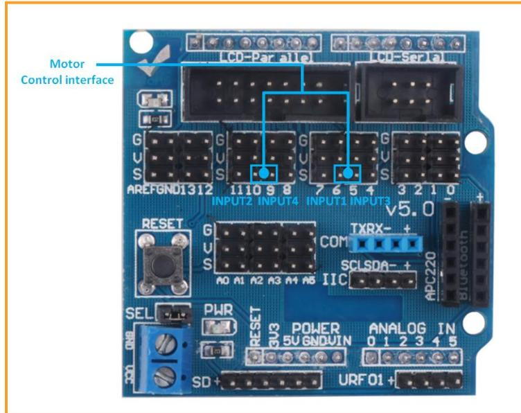
Figure.3.1.2.8 L298N and Arduino Expansion Board Connection Diagram
