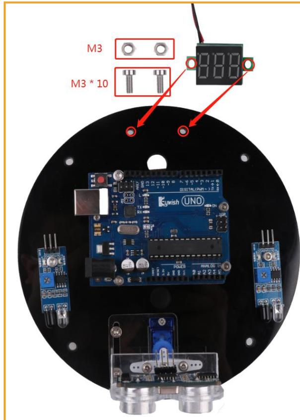
Figure 3.1.8.1 Schematic diagram of voltage display module installation
