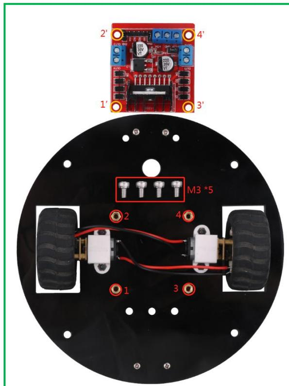
Note: Hole 1 corresponds to 1", hole 2 corresponds to 2", **tightened with M3\*5screw and so on**
