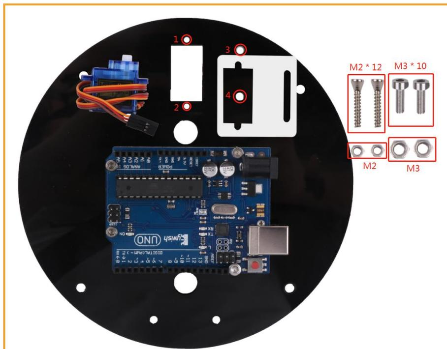
**Note: Firstly, place the servo base on the corresponding position of the acrylic plate and then put the servo and fix it with screws. The holes 1 and 2 are fixed with M2\*12 screws, and the 3 and 4 holes are fixed with M3\*10 screws.**
