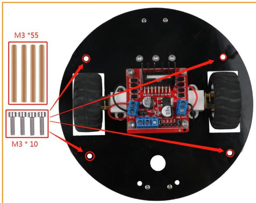
Figure 3.1.4.4 Schematic diagram of the installation of the upper acrylic plate pillar
