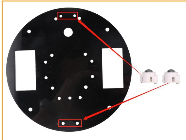
Note: The universal wheel is fixed by using its own two screws.
