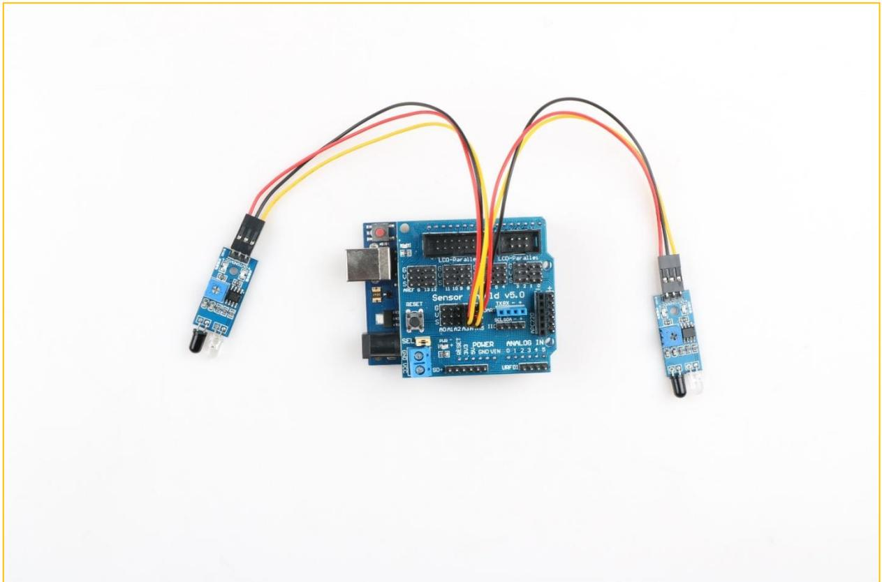
Figure 3.2.2.3 Connection of Arduino and Sensor
