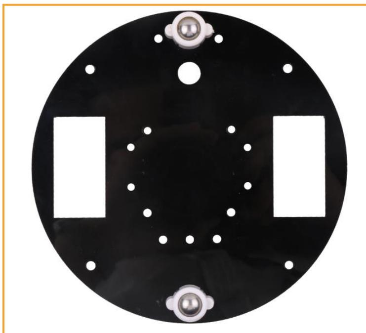
Figure 3.1.1.2 Effect diagram of the universal wheel installation
